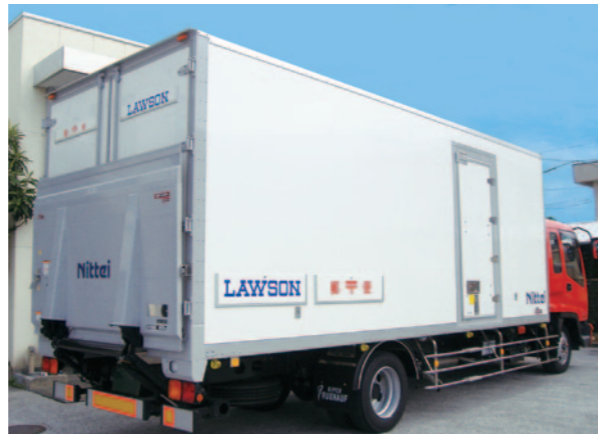
Temperature-controlled containers have been installed in Japan Post service trucks, which are used to deliver products refrigerated at different temperatures
