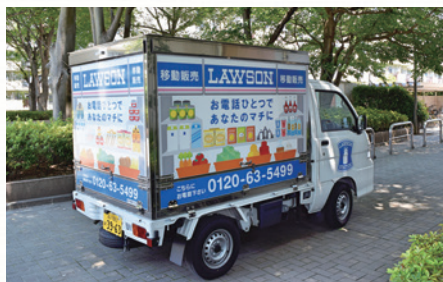
A new-type vehicle dedicated to mobile sales was introduced in November 2016. The truck has four different temperature sections to preserve food at suitable temperatures and is equipped with mobile POS devices that can register sales and print receipts.
