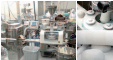
At the end of each day, machines are broken down and their individual parts carefully washed and disinfected.
