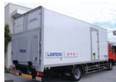
▲ Japan Post Service Co.,Ltd. delivery truck fitted with a temperature-controlled container to deliver products with different temperature requirements
