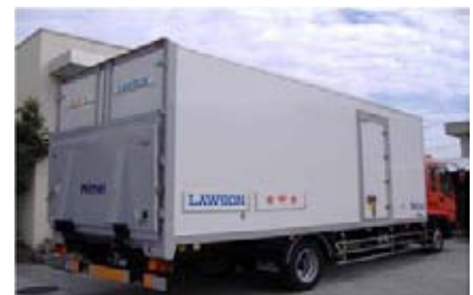
Japan Post delivery truck fitted with a temperature-controlled container to deliver products with different temperature requirements
