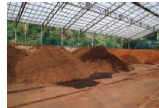
Bacteria is mixed into garbage to cause fermentation and decomposition into fertilizer.
