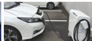
Changing the company car for the Supervisor (SV) to an EV made it possible to create a two-way power flow between the EV and the store by only connecting the EV to the EV charger with no need for in-store operation
