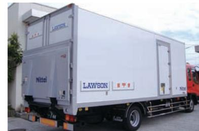
▲ Japan Post Service Co., Ltd. delivery truck fitted with a temperature-controlled container to deliver products with different temperature requirements
